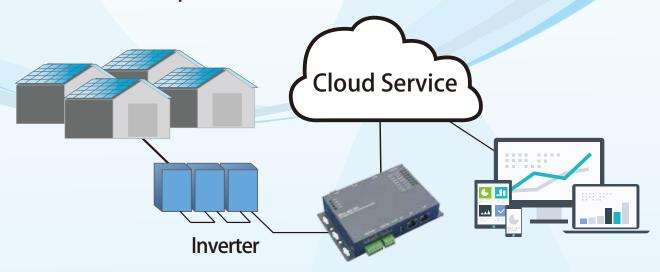
Transmit the solar power generation status to the cloud server, providing real-time power generation data and long-term record. Trace the immediate situation of each power plant through the cloud service.
